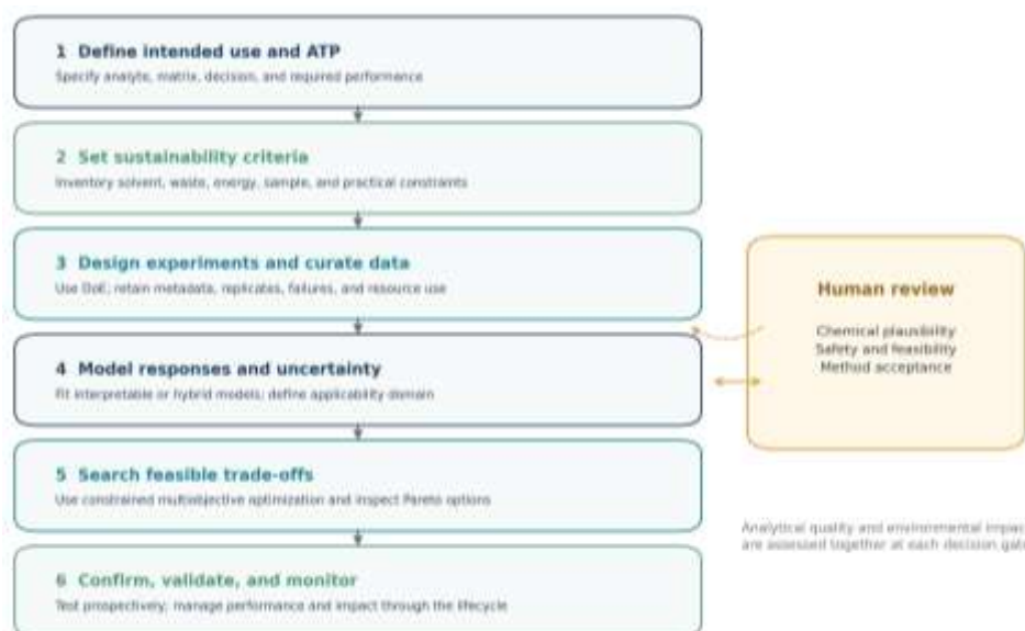
Fig 1: Integrated workflow for AI-driven green analytical method development. The schematic links intended use and the analytical target profile to a sustainability inventory, designed experiments,
