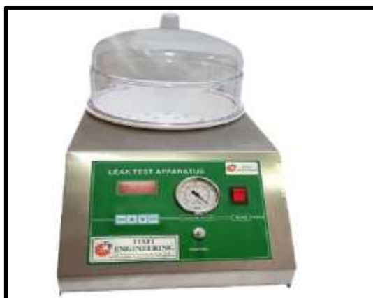
Fig 6: Leak test apparatus
