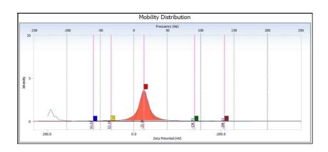
Zeta potential of nanoparticles of PS6 batch
