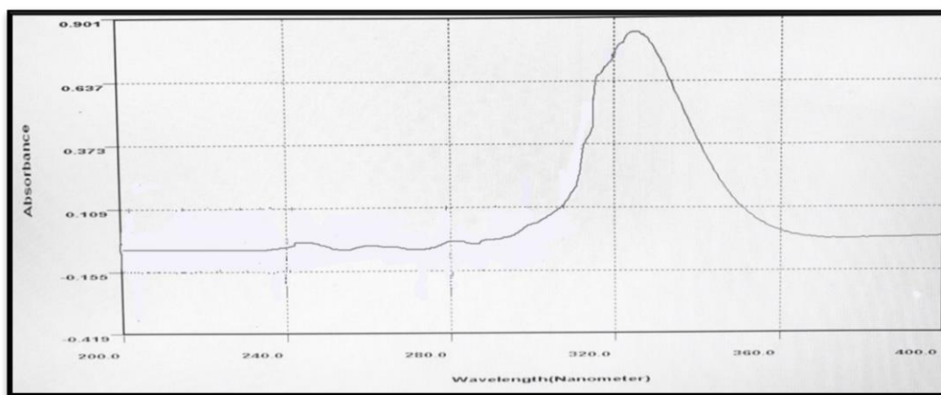
Fig No: 5 Absorption Spectrum of Lurasidone
