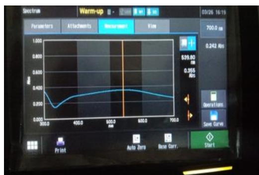
Fig: 2 UV- Visible spectron of Ag Nanoparticles, synthesized by reducing \text{AgNO}_3 using ethanolic extract of justicia Adhatoda [EEJA]
