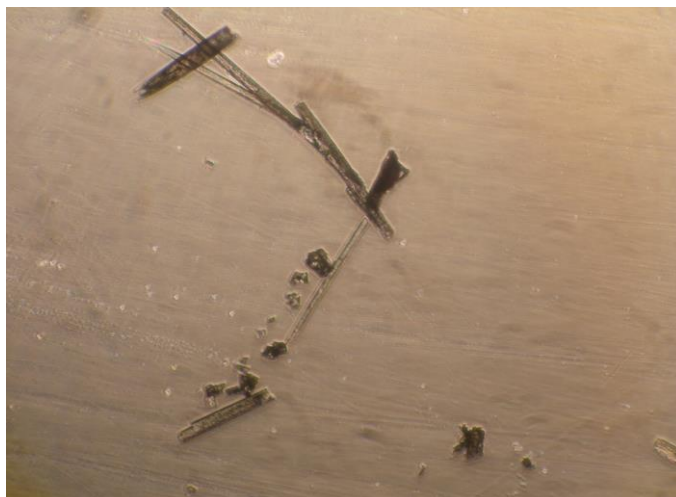
Fig 3: Spiranolactone-Succinic acid co-crystal at 45X magnification
